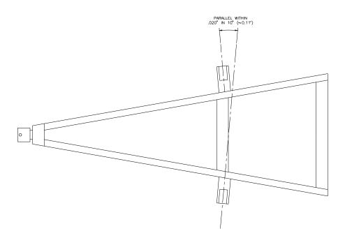
Toe-in / toe-out is unpredictable and cannot be summarized in a table like orientation errors. Many factors contribute to the phenomena including the type of load cell installed, the amount of misalignment, the test surface, etc. As mentioned above, the best method for minimizing its effects is using proper fixtures.
