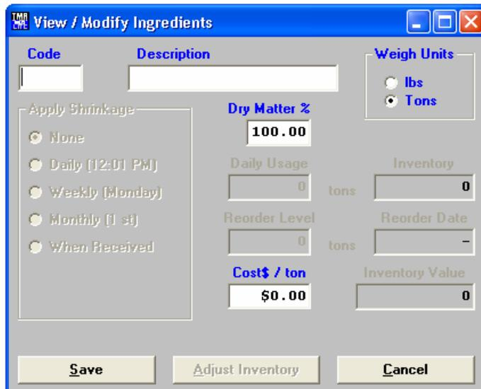
Each ingredient will be assigned an ingredient code. This code is displayed as an operator prompt on the scale and remote. Please limit the code to 6 characters. For example: Corn silage may have an ingredient code of SILAGE or CORNSI. Enter the ingredient description, weigh units, dry matter percentage and click Save.
