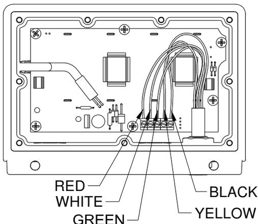
5. Place the wires in their correct locations as marked on the circuit board and tighten the screws on the terminal blocks securely.
