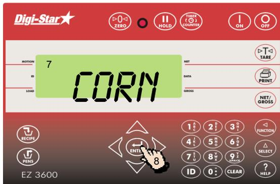
7. The weighing indicator displays the name and amount of the ingredient to be loaded. As soon as the ingredient is loaded, the weighing indicator will count down to zero.
