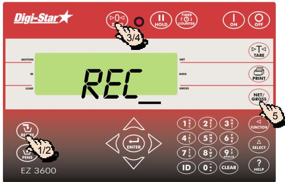
1. Press and hold until the weighing indicator emits a high pitched signal and *PROGRAM* and the first recipe number are displayed in succession.
