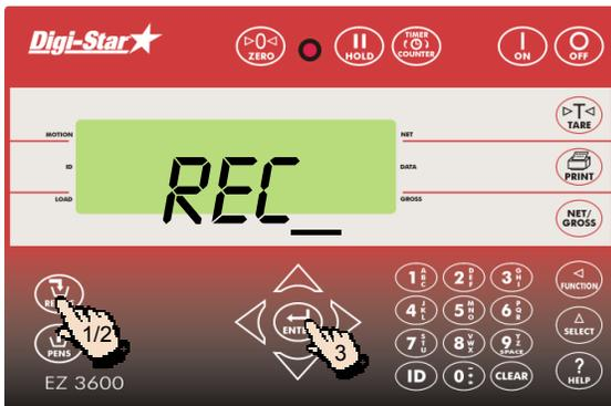
1. Press and hold until the weighing indicator emits a high pitched signal and *PROGRAM* is displayed.
