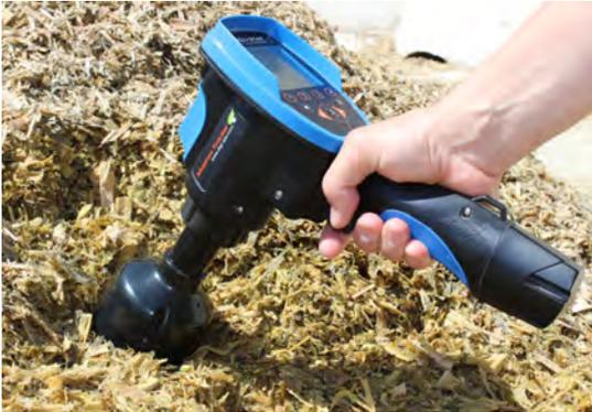
A hand-held NIR scanning device that rapidly measures the DM and moisture content of animal feeds. The Moisture Tracker™ device provides livestock producers with near instantaneous, accurate DM and moisture readings which enable livestock producers to quickly react to changes in DM thus ensuring that the ration delivered matches the ration calculated.
