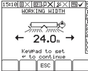
Using the number keypad, the width can be programmed and then confirmed using the
