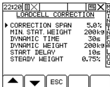
On this screen the technician can configure the operation of the load cells for calibration purposes.
