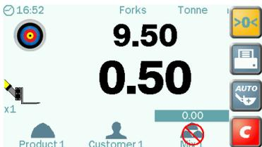
1. Lift the load up to the weighing position. The alarm will sound one beep and the “live” weight will be displayed. Keep the loader as steady as possible while the weight is taken.
