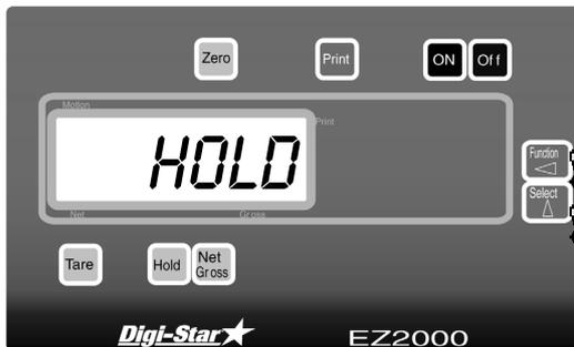
The FUNCTION key provides additional features to the operation of the scale. The FUNCTION key is similar to the F1 key of a computer. The SELECT key is used to determine what operation will occur when the FUNCTION key is pressed.
