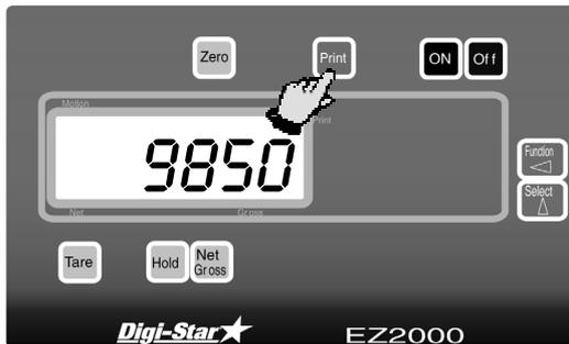
Press the **Print** key. Scale data will be sent to the printer.
