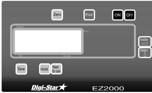
To exit setup without changing any values, press and hold the **Tare** key, then press the **ON** key.
