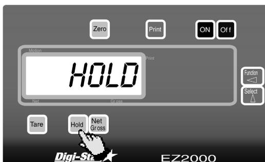
**HOLD mode prevents the displayed weight from changing due to "zero shift" while moving the scale. Use of this mode is optional.**
