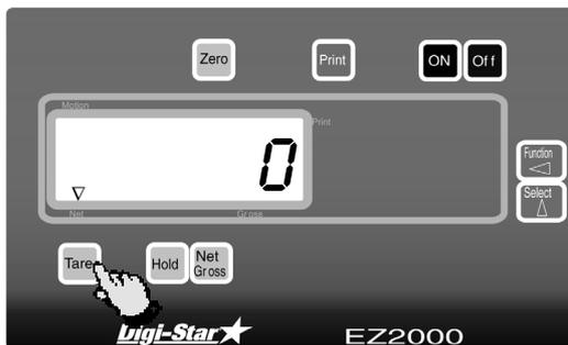
**NET mode displays the weight change after a TARE has been performed. TARE creates a temporary zero at that weight value.**
