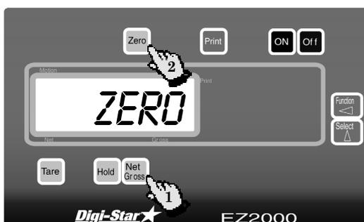
Press **Net Gross** and then within three seconds, press **Zero**.
