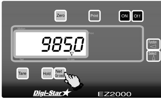
**GROSS mode displays the weight change since the unit was last Zero/Balanced.**
